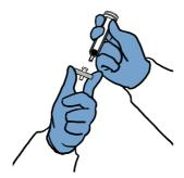
✓ Pre-saturate filter (see Section A10) and return filtrate back to vessel
