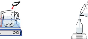
Weigh 452.3g (450 mL) of "Concentrated FaSSIF" into a container for each dissolution vessel
