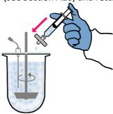
✓ Filter and collect remaining dissolution sample (about 1mL) for analysis
