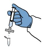
Discard filter, re-attach syringe to cannula
